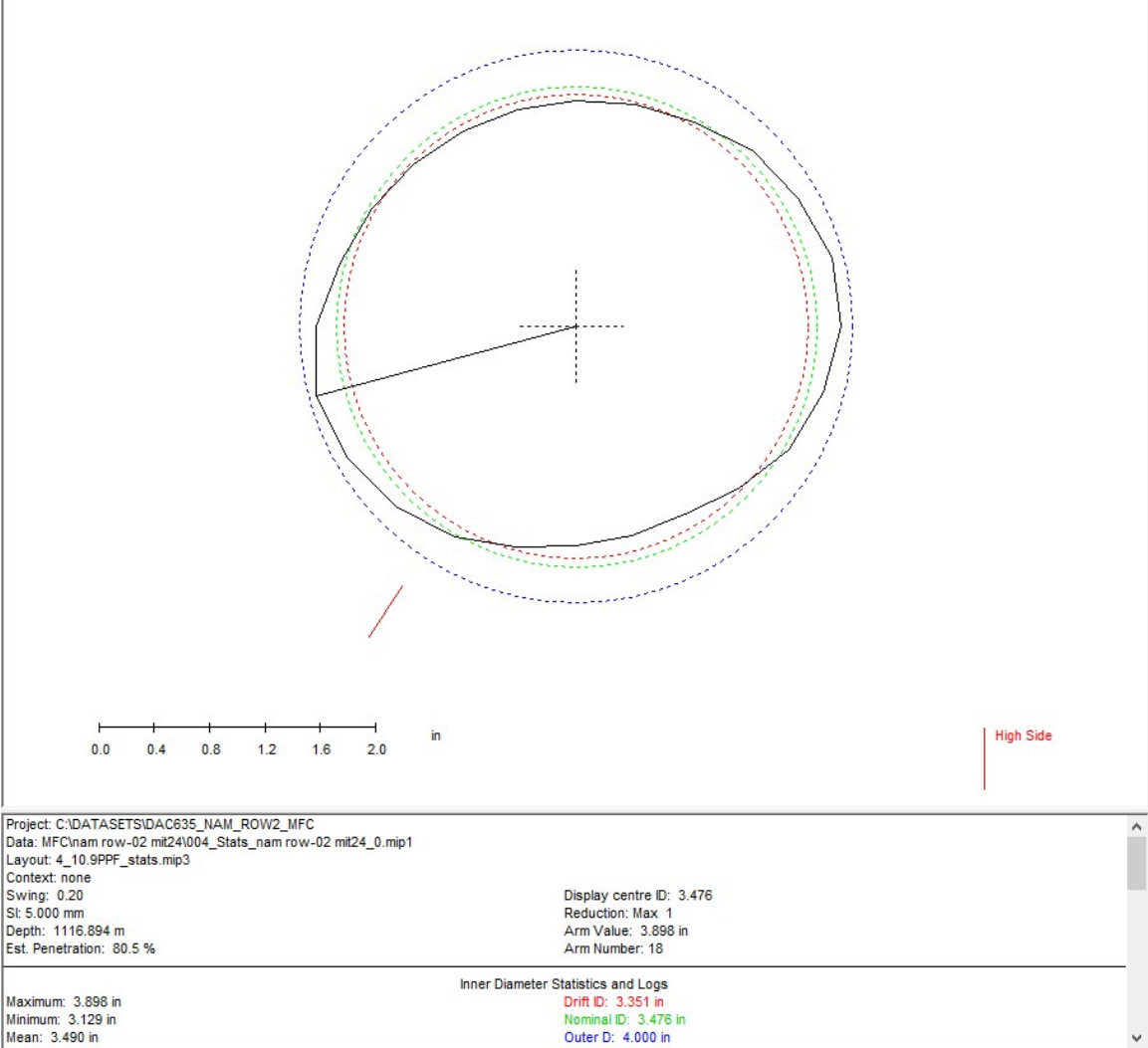
Figure 6: Maximum Recorded ID within 4", 10.9 lb/ft Tubing (Cross-section)
