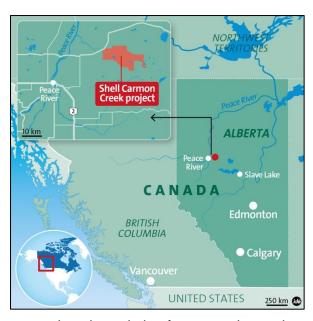
The Shell Carmon Creek Project, under construction, will produce up to 80,000 barrels per day of oil using enhanced oil recovery methods, where steam is injected into the underground reservoir to help produce the heavy oil. The water co-produced with the oil recovered underground will be treated and re-used to generate steam. This approach maximizes the amount of process water recycled (approximately 99%).
