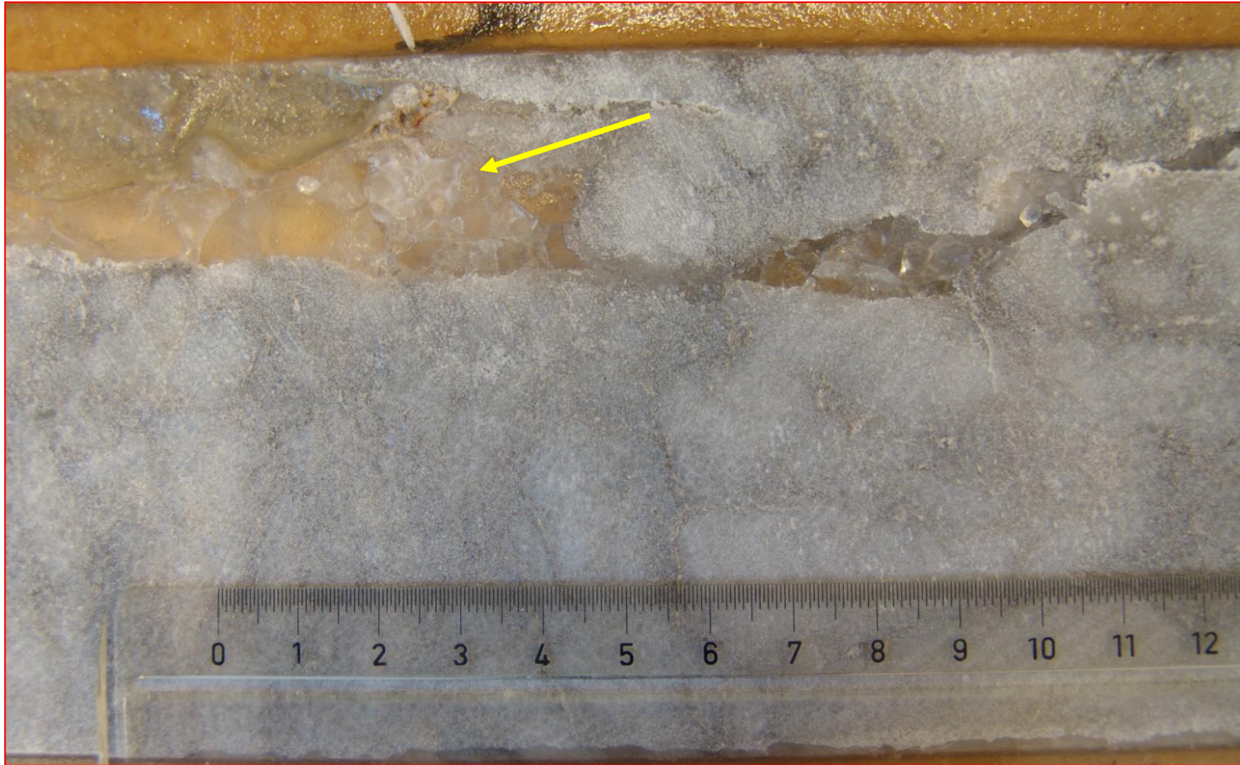
Figure 15. Tubberaen-7. 1490.8m AH. ZEZ2A. Halite filled fracture (arrow) in Anhydrite.
