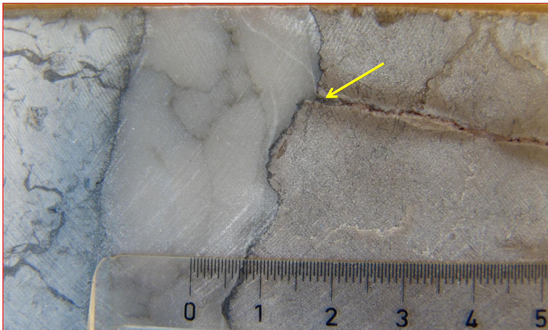
Figure 11, Rossum Weerselo-5 1195.8 ZE3C. Partly open fracture (+/- 1mm wide) in Dolomite abutting at lithology change to Anhydrite (arrow).
