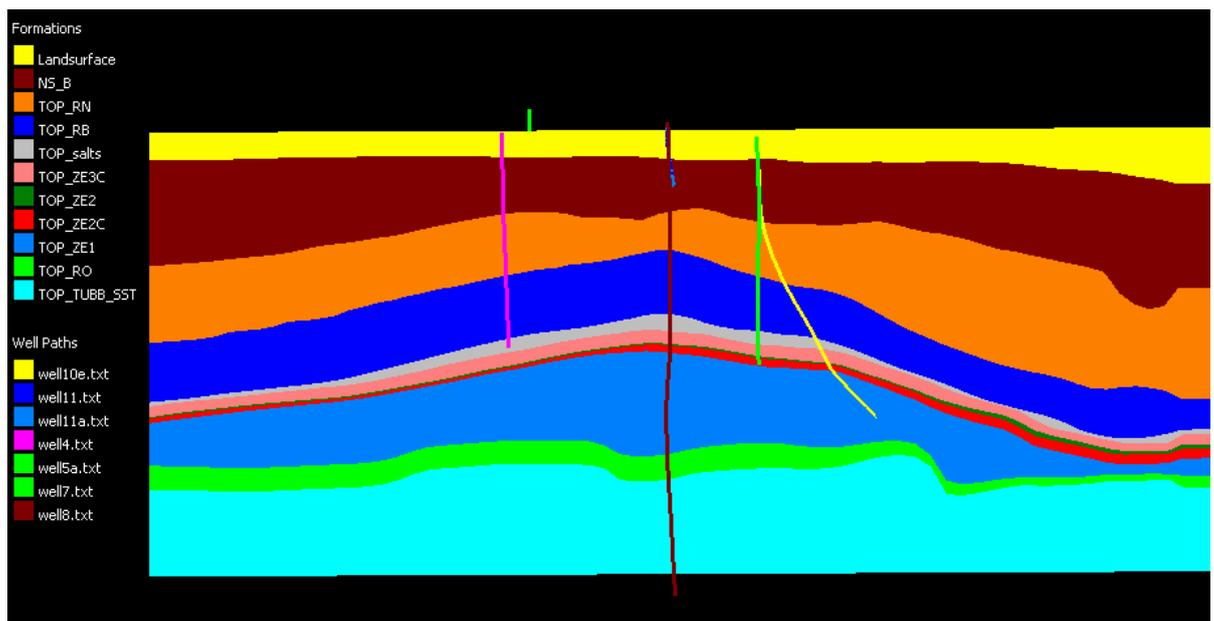
**Figure 2.1: Geology of the Tubbergen static model (as Geomec mesh cross section) used to construct the dynamic Dynamo-MoReS simulation model and. Formations of interest include the Zechstein 3 Halite (TOP\_salts: grey), the Zechstein 3 Carbonate (TOP\_ZE3C: pink), the Zechstein 2 Halite (contained within the TOP\_ZE2 interval along with ZE22 Anhydrite and ZE23 Grey Salt Clay: dark green), and the Zechstein 2 Carbonate (TOP\_ZE2C: red).**
