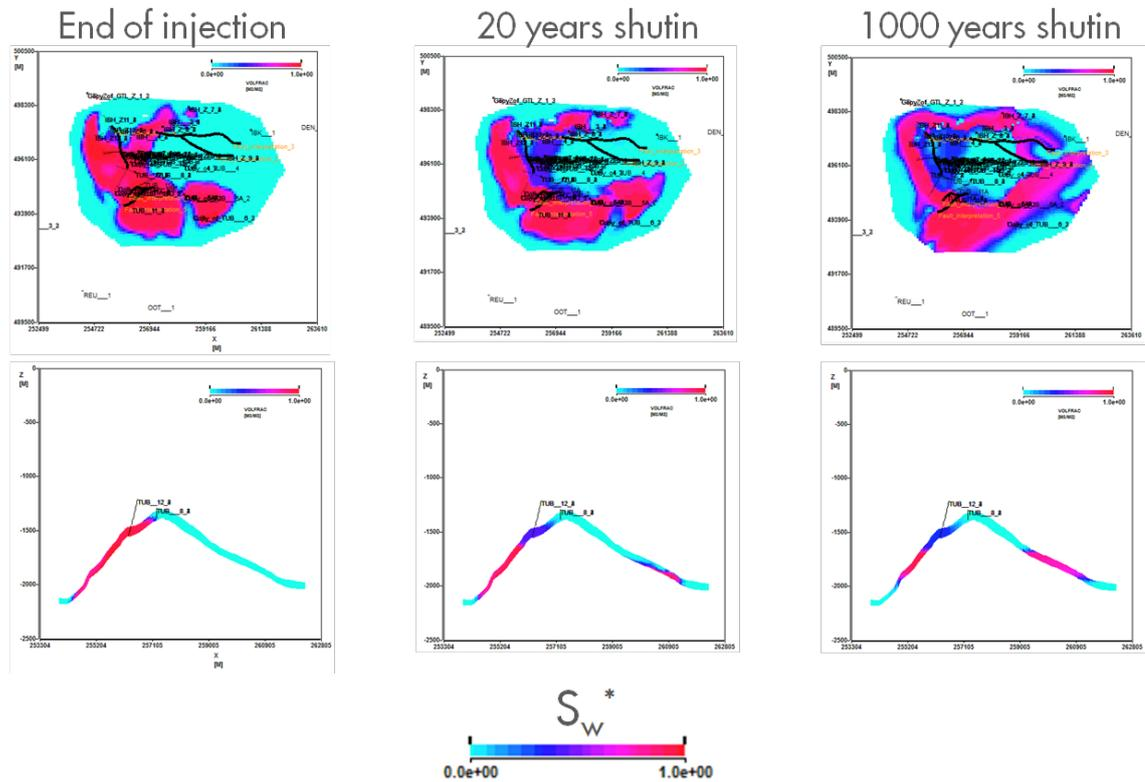
**Figure 3.1:** XY and XZ slices through the full field model showing the fresh water fraction of the total water saturation ( $S_w^*$ ) distribution after 20 years (end of injection), 40 years (20 years shut in), and 1020 years (1000 years shut in).  $S_w^*$  is defined as the water saturation multiplied by the injection water tracer concentration.
