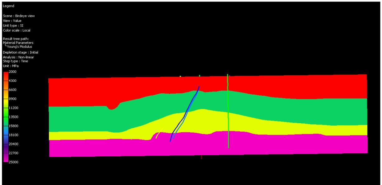
Figure A2: Young's Modulus on cross section, ranging from 2 to 25 GPa.
