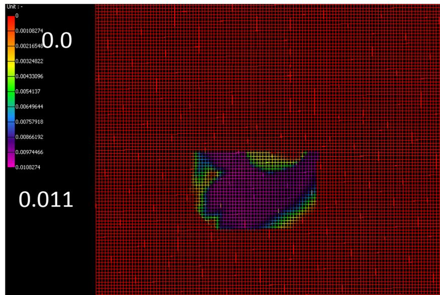
**Figure 3.5: Concentrated salt dissolution (shrinkage strain) for the same total amount (painted on mesh).**
