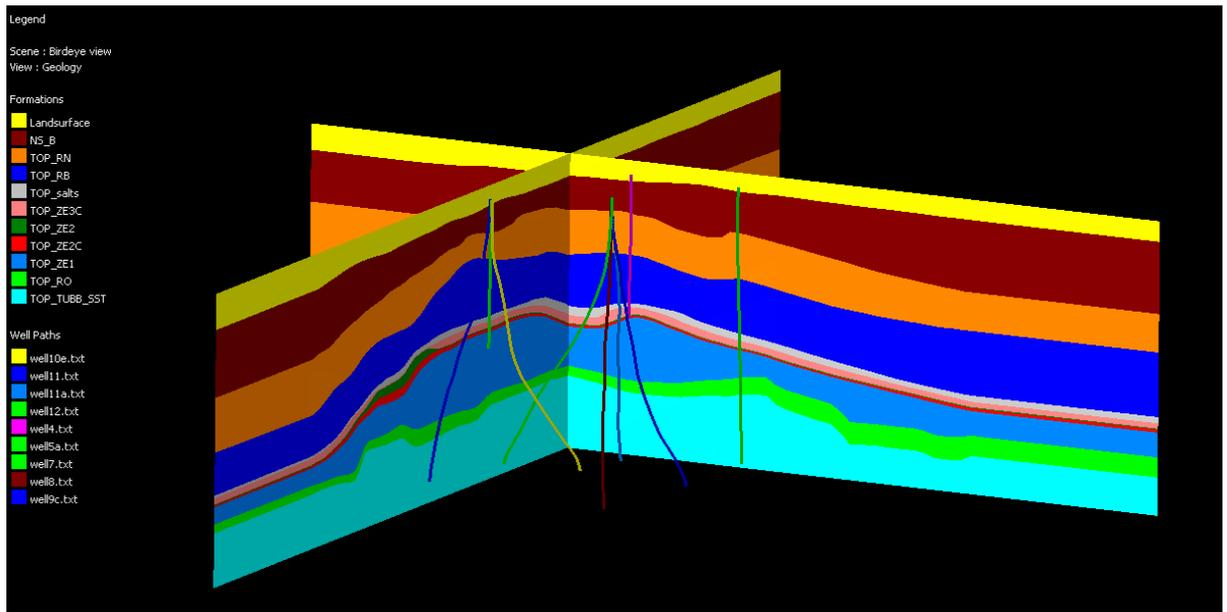
**Figure 2.3:** Geology of the Tubbergen static model (as Geomec mesh cross section) given two cross sections and some wells, some crossing the reservoirs.
