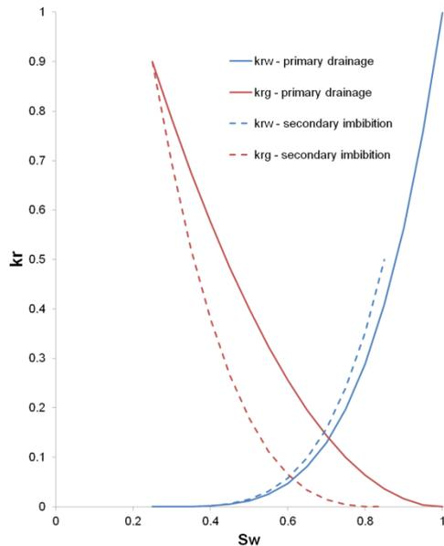
**Figure 2.2: Corey-Model primary drainage and secondary imbibition relative permeability curves used in this study (input parameters are summarised in Table 2.2).**
