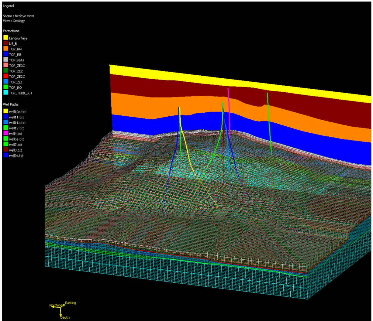
**Figure 2.5:** Cross section and partial mesh (salt, carbonates and underburden) with some wells for orientation. The surface (lateral) mesh is 100x100 m. The vertical size of the elements varies per location (depending on layer thickness).
