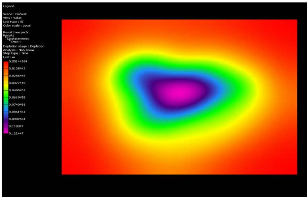
**Figure 3.4:** Subsidence bowl (0-12 cm) resulting from salt dissolution and salt creep leaving zero brine volume in the salt.
