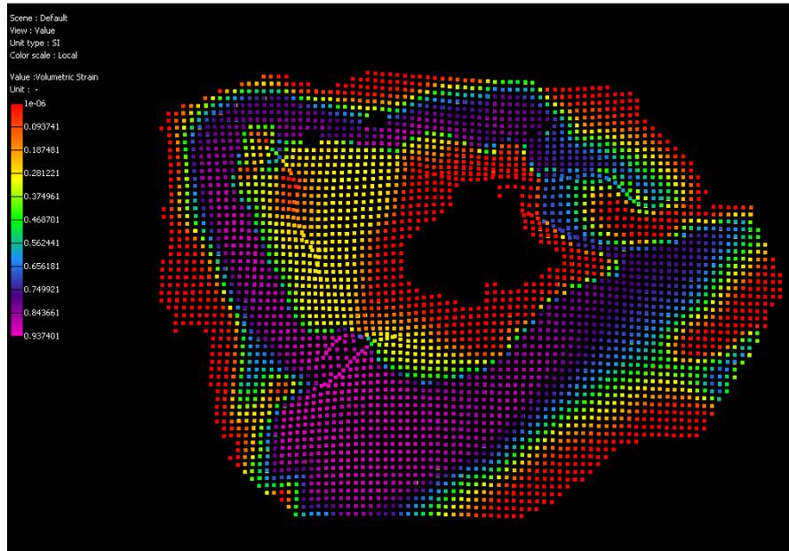
**Figure 3.2:** Total water saturation change ( $S_w$ ) distribution after 1000 years shut in, used to predict salt dissolution. The purple area is the area of fresh water injection. In the middle, there is still a high gas saturation and at the edges, the water (brine) saturation was initially high.
