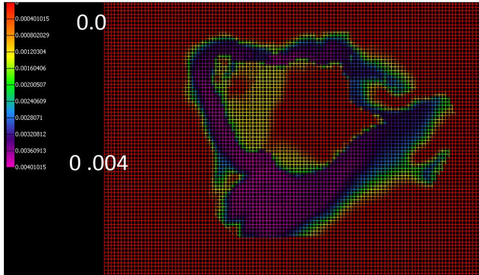
**Figure 3.3:** Shrinkage strain assigned to the carbonate to represent the salt dissolution volume.
