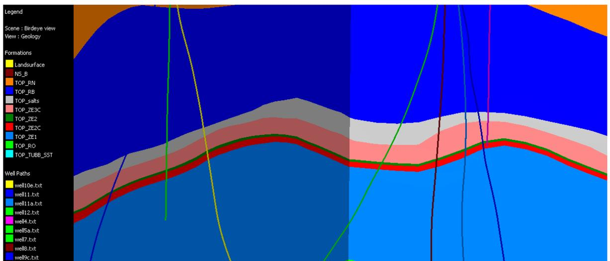
**Figure 2.4:** Zoom in on cross sections with crestal properties of layer thicknesses. The grey layers is the top salt cap. The pink and red layers are the carbonate reservoirs ZE(Z)3C and ZE(Z)2C
