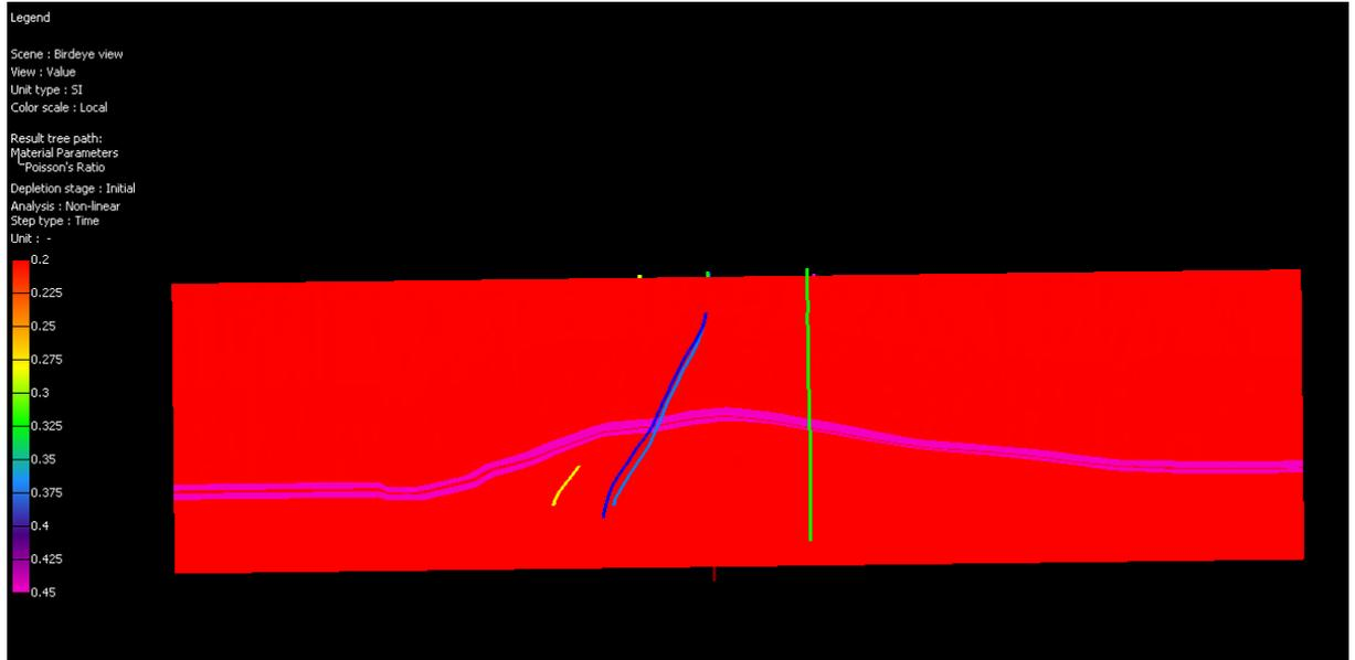
Figure A3: Poisson's ratio on cross section, constant at 0.2 for all the rocks except the carbonates. Carbonate Poisson's ratio is 0.45 to force the contraction strain (from salt dissolution) to end up in subsidence .
