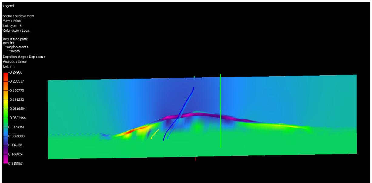
Figure A4: Vertical displacement (subsidence) on a cross section. The red/yellow parts are upheave of the under burden, whereas blue is subsidence of mainly the overburden.
