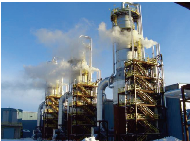
FIGURE 5: 3,000 gpm produced water evaporator system at suncor firebag.
